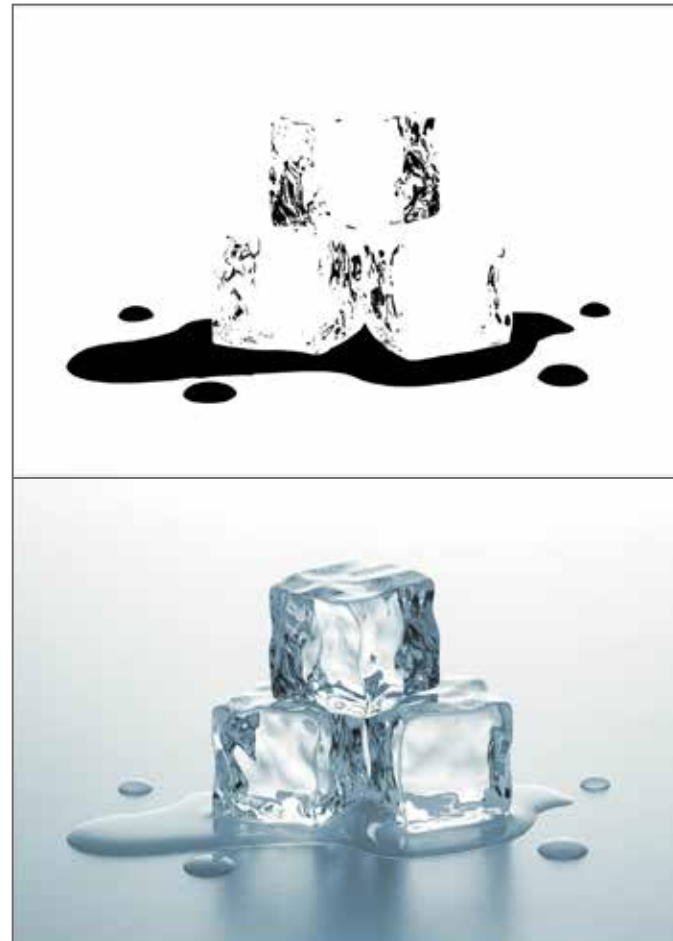
The top image shows the separation of the specific area where spot coating will be applied to the bottom image.
